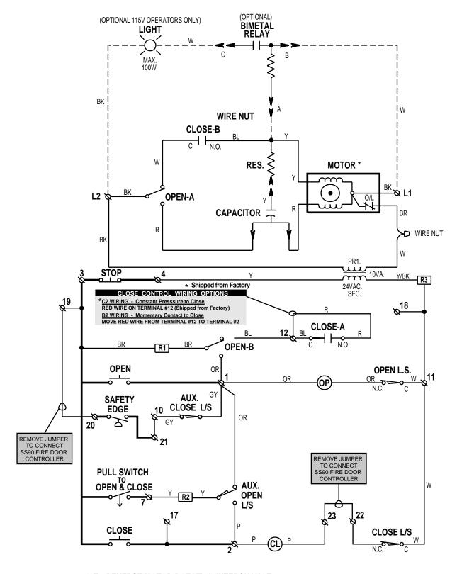
\* TO REVERSE MOTOR ROTATION INTERCHANGE RED AND YELLOW MOTOR WIRES.
