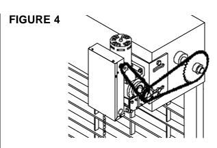
**IMPORTANT:** The shelf or bracket must provide adequate support, prevent play between operator and door shaft, and permit operator to be fastened securely and with the drive shaft parallel to the door shaft.
