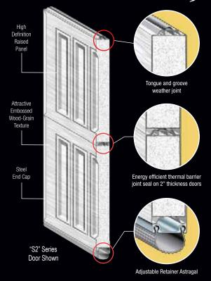
The beauty of the Therma Classic is more than skin deep. Therma Classic is built with Northwest Door's time proven sandwich-type construction method. Interior and exterior galvanized and prepainted steel skins are pressure laminated to a 2" thick CFC-free (EPS) polystyrene core forming a continous bond. A flexible joint seal is added to the tongue and groove section joints which seal and also provide a true and natural thermal break. It's construction is both fire and smoke rated.
